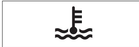
When the ignition switch is turned to the "ON" position, this light comes on briefly so you can check that the light is working. If this light blinks while driving, it means the engine is running hot. Avoid driving conditions that may lead to actual overheating. If the light stays on without blinking, then the engine is overheating. Follow the instructions in the "If the Engine Overheats" of "EMERGENCY SERVICE" section.
