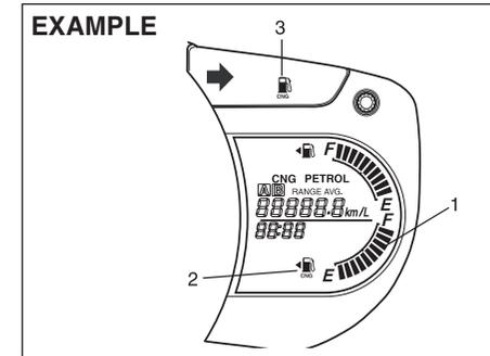
CNG level indicator (1) is built into the display. When the ignition switch is in the "ON" position, this gauge gives an approximate indication of the quantity of fuel in the CNG tank. "F" stands for full and "E" stands for empty.
