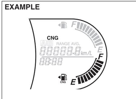
This is emergency mode and may be used in cases where there is no petrol in petrol tank. In this mode vehicle starts in CNG mode and continues running in CNG mode. With ignition "ON" and engine not running, press and hold the changeover switch till only CNG indicator is displayed. In this mode, CNG indicator is displayed and Petrol indicator remains "OFF".
