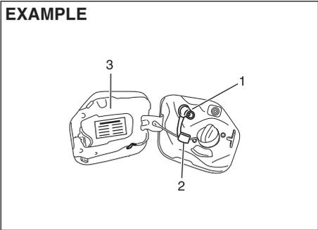
The CNG filler valve is integrated in fuel box next to petrol filling area.
