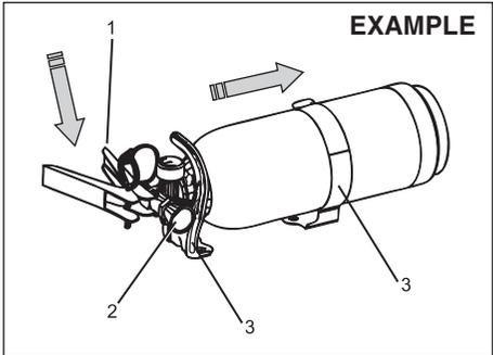
Insert the body of fire extinguisher (1) in to the clamps (3) and place the nozzle (2) carefully downwards.
