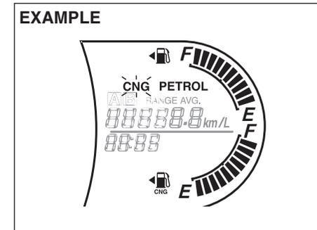
In this mode engine starts in petrol mode and then automatically changes to CNG mode after reaching programmed warming up condition. With ignition switch ON and vehicle started in "AUTO MODE", CNG indicator blinks on the display and PETROL indicator is displayed. After changeover to CNG, CNG indicator will be displayed and Petrol indicator will switch OFF automatically.
