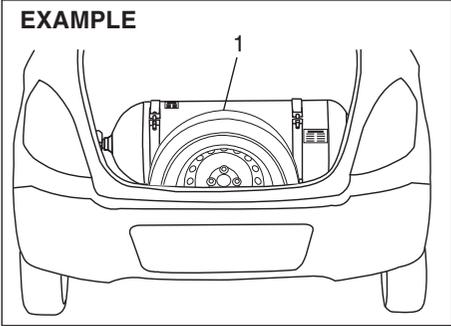
Spare wheel is located behind the CNG cylinder and secured with help of a mounting knob.
