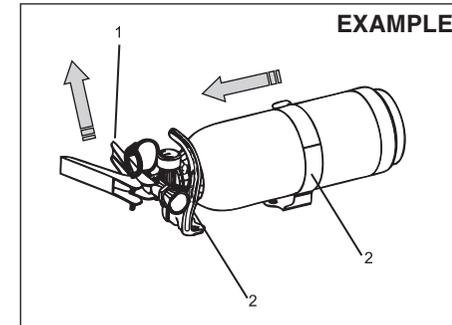
Lift Lever (1) of fire extinguisher slightly upwards and pull the fire extinguisher in the direction as shown in the figure, in order to disengage it from clamps (2).
