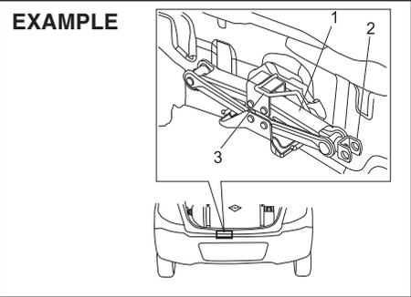
Jack (1) is located between spare wheel and vehicle rear as shown in the illustration.
