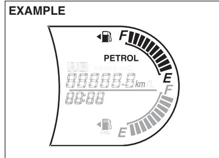
In this mode vehicle starts in petrol and continue running in petrol mode. In this mode, petrol indicator is continuously displayed and CNG indicator will remain "OFF".
