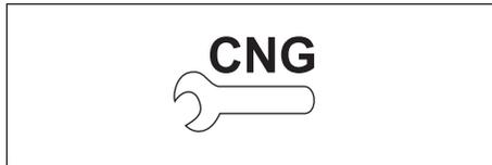
When the ignition switch is turned "ON", this CNG malfunction warning lamp comes on briefly, to check that the CNG malfunction lamp is troublefree.
