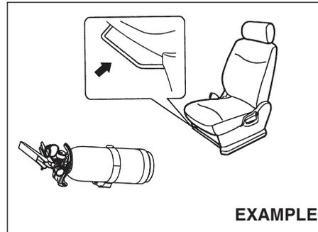
Fire extinguisher is located below co-passenger's seat.
