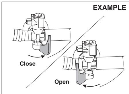
CNG supply can be switched off by closing the manual shut-off valve.
