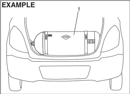
CNG cylinder (1) is installed in the luggage compartment.
